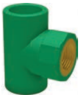
G 8130gB PP-RCT-RG Ü-T-Stück 90° IG-zyl grün PP-RCT-Bronze Transition-Tee 90° female-thread-cyl green
